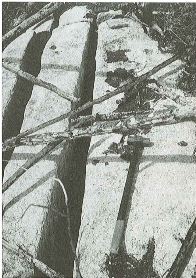
Plate 13. Slab-like outcrop blocks of coarse-grained red granite at a small outcrop northeast of the Red Cliff transmission tower. Although unsuitable for large tile blocks, these may be of interest for monument slabs.
