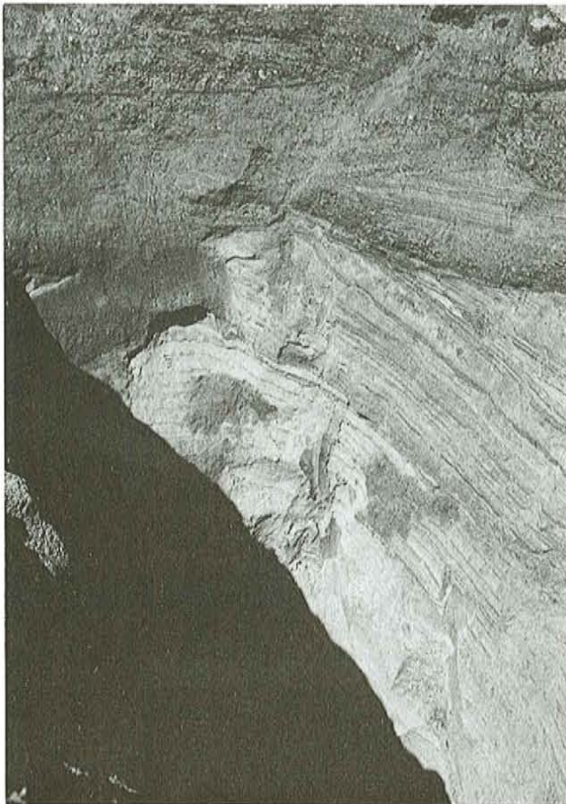
Plate 4. Excavator dug test pit in sand, note dark banding of heavy minerals.
