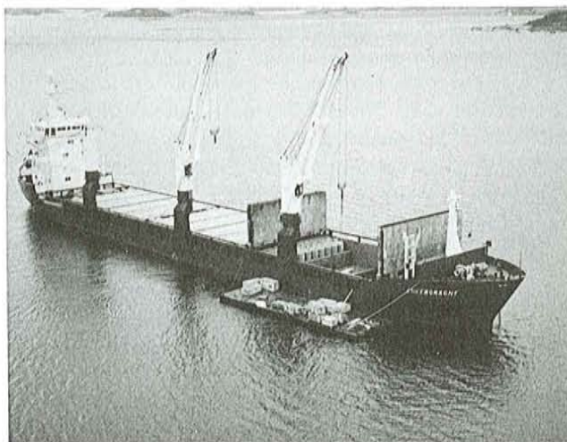
Plate 3. Loading blocks of anorthosite onto a transatlantic vessel near Ten Mile Bay.
