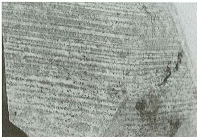
Plate 1. Photograph of highly flattened and welded amphibole ash-flow tuff (subunit 5d) from the Bartletts Creek ring-dyke locality.
