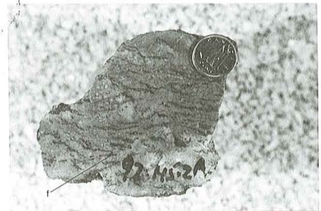
Plate 2. Photographs of silica-sulphide alteration; a (top left)—hand specimen of silicified pebbly conglomerate with disseminated chalcopyrite; b (top right)—polished section showing chalcopyrite and pyrrhotite in a silicate gangue. Reflected light; field of view—2 mm.; c (left bottom)—highly silicified, intensely deformed rocks with sulphide veinlets (black) folded and transposed into the plane of foliation. Rootless fold indicated by 'f'; d (right bottom)—photomicrograph of folded sulphide laminae (black) in silicified conglomerate; field of view—2 mm, crossed polars.
