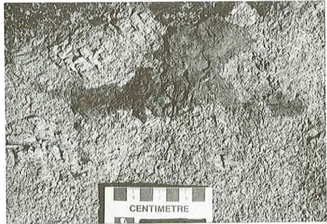
Plate 8. Coarse- to very coarse-grained patch of subequant plagioclase laths and anhedral olivine and magnetite (darkest grey) in a medium-grained anorthosite groundmass.
