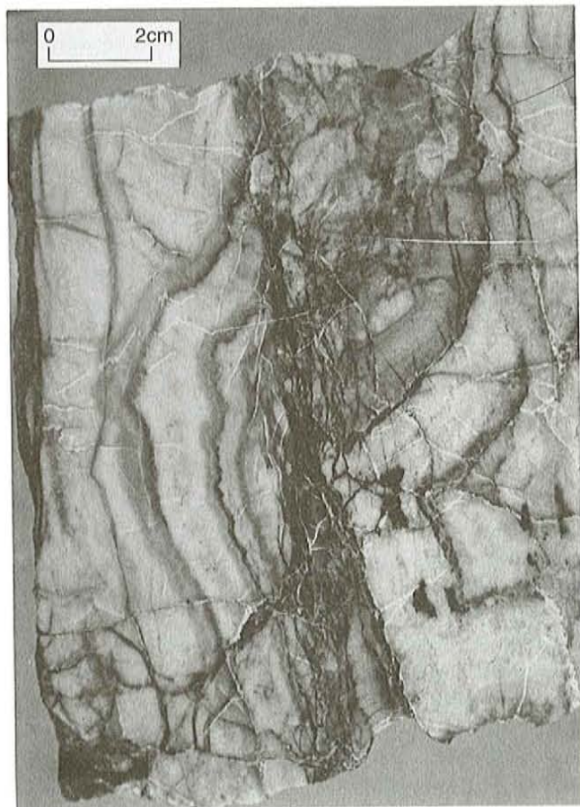
Plate 10. Auriferous (2 g/t Au), banded quartz-K-feldspar-hematite ("low-sulphidation"-style) veins, Avalon High-Alumina Belt, near Manuels.
