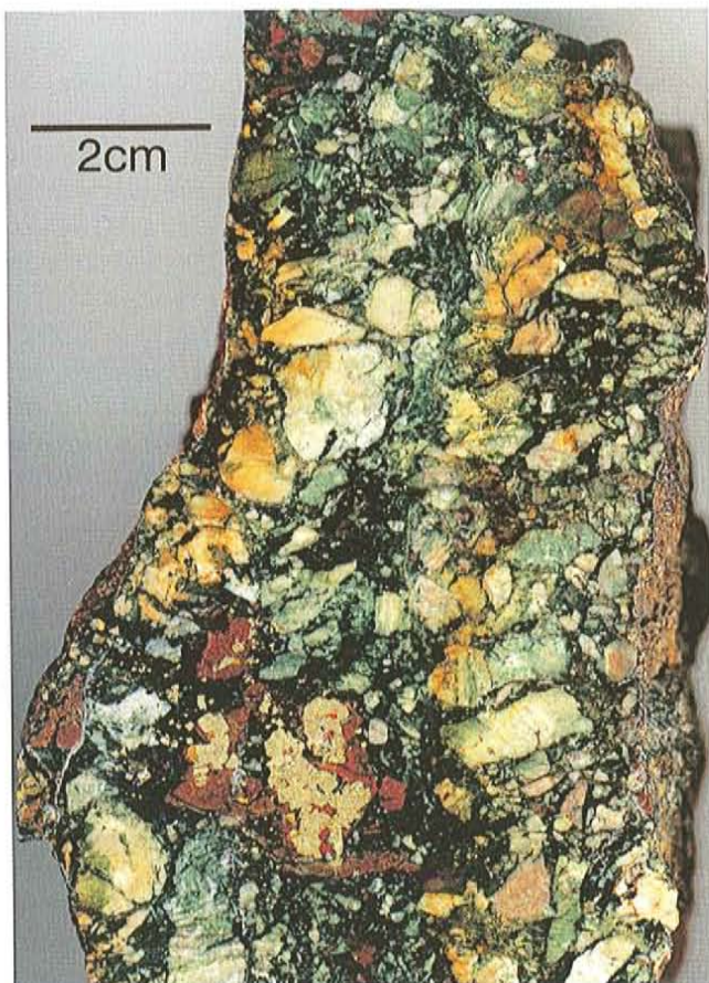
Plate 3. Au-Ag-As-bearing chlorite-rich hydrothermal breccia (11.2 g/t Au, 210 g/t Ag), with pyrite and hematite in the matrix; Roadcut prospect.
