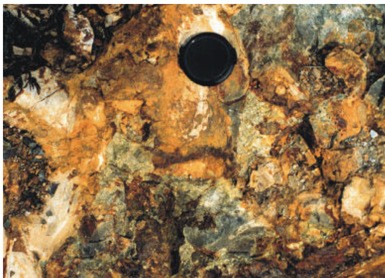
Plate 2. Mineralized auriferous breccia at the Lodestar prospect. Visible mineralization consists of pyrite, arsenopyrite, chalcopyrite and magnetite.
