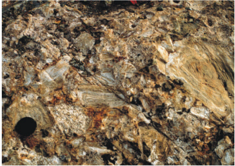
Plate 3. Breccia at the Lodestar prospect containing clasts of gabbro, sedimentary rocks, diabase and quartz–feldspar porphyry. Note alteration rims in some sedimentary clasts.
