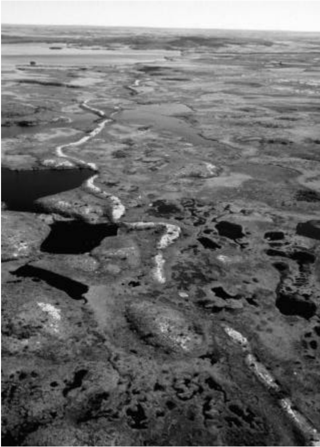
Plate 4. East–west-trending esker on the western part of the Tug Pond map area. These features indicate westward retreat of late Wisconsinan ice and also provide excellent sources of granular aggregate.
