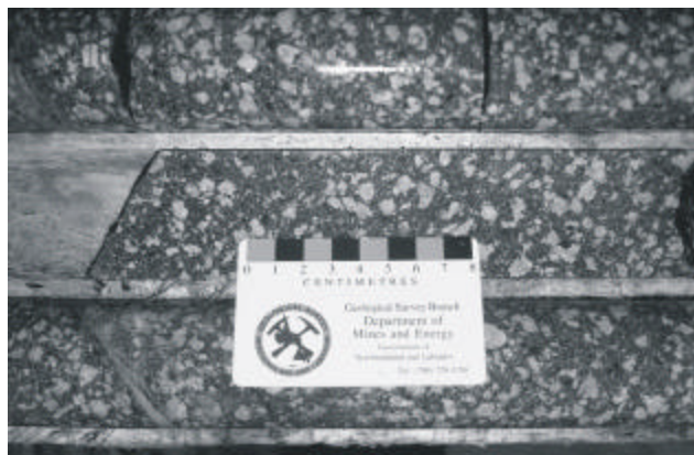
Plate 6. Light green to grey, medium-grained, massive K-feldspar phenocrysts set in a groundmass of fine-grained rhyodacite.
