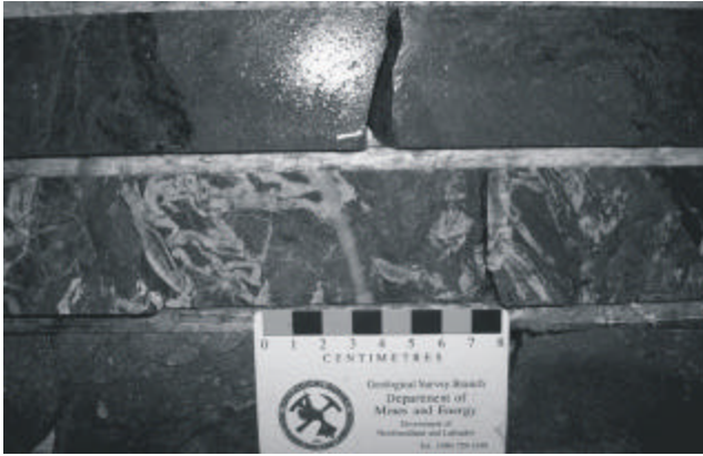
Plate 3. Intense carbonate and chlorite alteration in dominantly pyrite mineralized felsic volcanic rocks.
