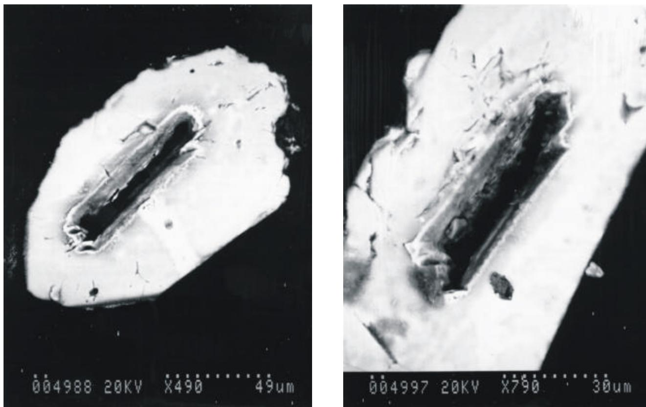
**Plate 4.** *Scanning electron micrographs showing line raster-ablation pit in zircon crystal.*
