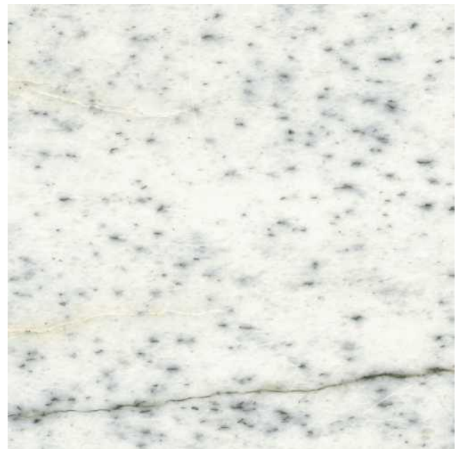
Plate 11c. Polished slab of white, graphitic marble from a stream, 11 km east-northeast of Coal Brook, southwest Newfoundland, cut across the foliation.
