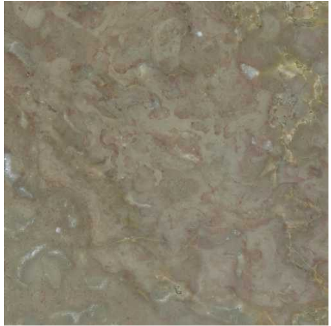
Plate 5b. Polished slab of Flower's Cove dolostone, cut parallel to the laminae.
