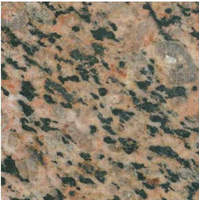
Plate 2c. Polished slab of Cartwright granite, cut across the foliation.
