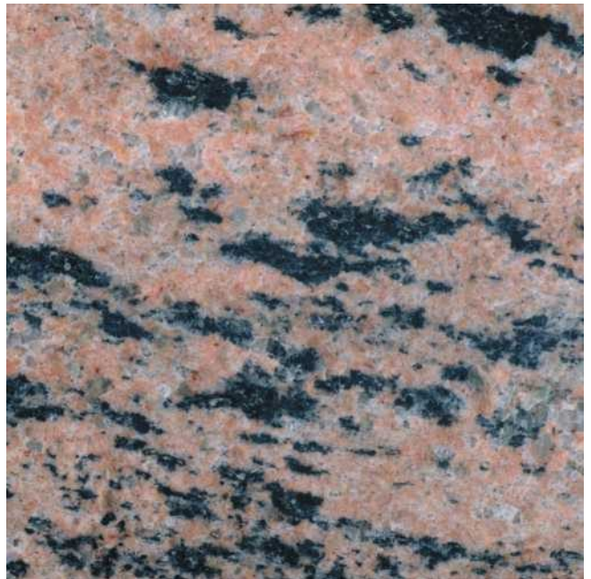
Plate 9c. Polished slab of wispy-banded gneiss from the area west of Sop's Arm, cut across the foliation.
