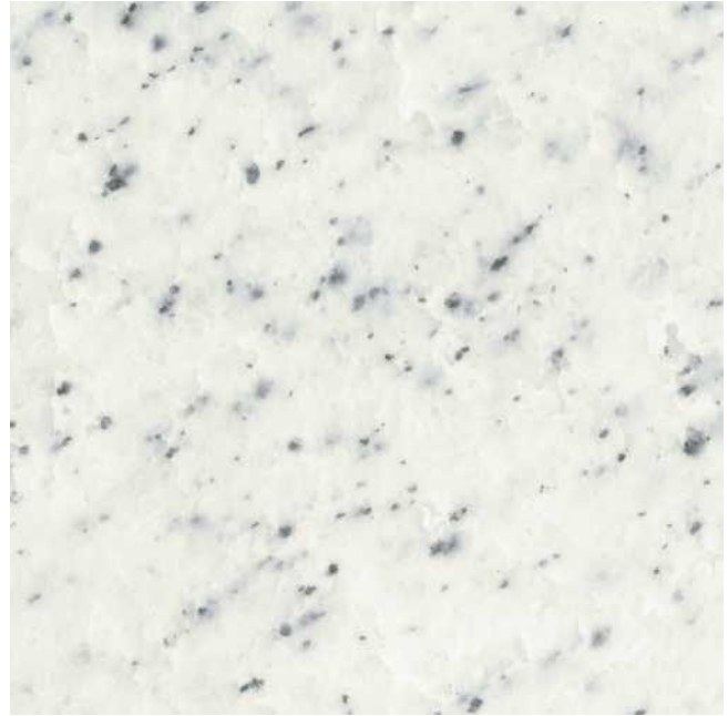
Plate 11b. Polished slab of white, graphitic marble from a stream, 11 km east-northeast of Coal Brook, southwest Newfoundland, cut parallel to the foliation.
