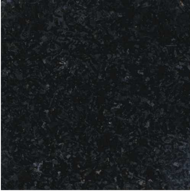
Plate 1b. Polished slab of black gabbro from aggregate quarry, east of Ossokmanuan Lake.
