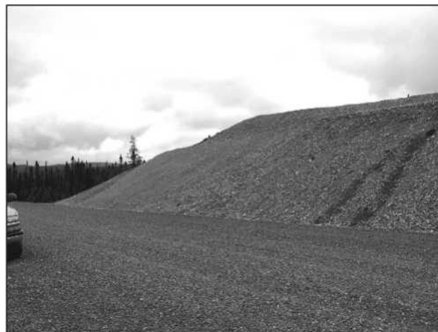
Plate 4. A 10-m-high sandy gravel exposure along roadcut in NTS map area 13H/6 (Zone 1, Deposit 4).
