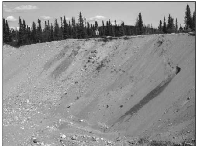
Plate 2. A 10-m-high gravelly sand exposure in abandoned quarry along the south boundary between NTS map areas 13H/3 and 13H/4 (Zone 1, Deposit 2).
