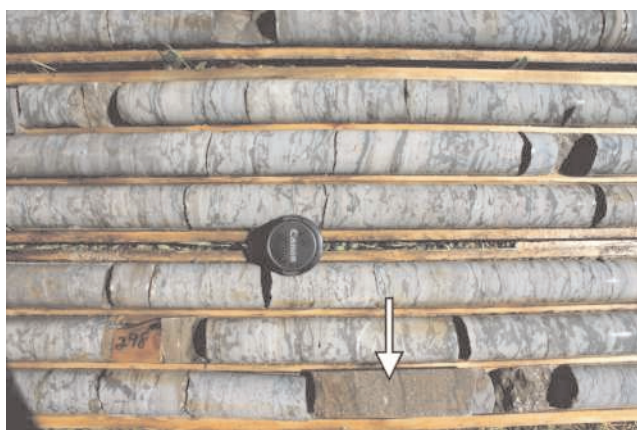
Plate 8. Bioturbated dolomitic limestone from the Lower limestone, Catoche Formation, DDH RND 001, Port au Choix Peninsula. The slabbed core in the lowest run (arrow) is an intraclastic, skeletal grainstone bed. Lens cap is 6 cm diameter.
