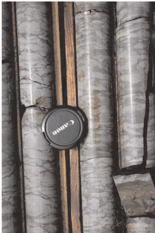
Plate 27. Stylonodular, dolomitic lime mudstone-wackestone of the Upper limestone member, Table Point Formation, DDH RND 001, Port au Port Peninsula. Lens cap is 6 cm diameter.
