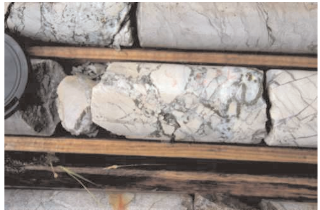
Plate 24. Brecciated dolostone, Aguathuna Formation, just below the St. George Unconformity, DDH RND 002, Port au Port Peninsula. Isopachous pyrite coats clasts in the breccia. Lens cap is 6 cm diameter.
