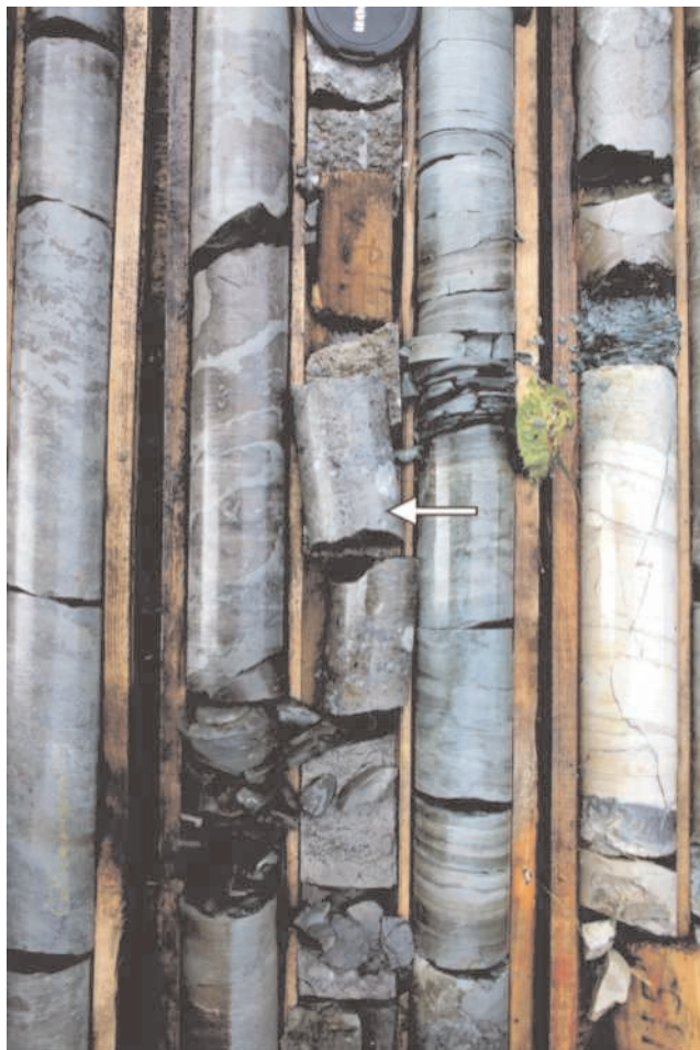
Plate 26. Basal conglomerate (arrow, middle core), Spring Inlet Member, Table Point Formation, DDH RND 002, Port au Port Peninsula. Underlying dololaminite and shale of the Aguathuna Formation occurs in the core to right and overlying nodular Table Point Formation limestone marks the core to left. Lens cap is 6 cm diameter.
