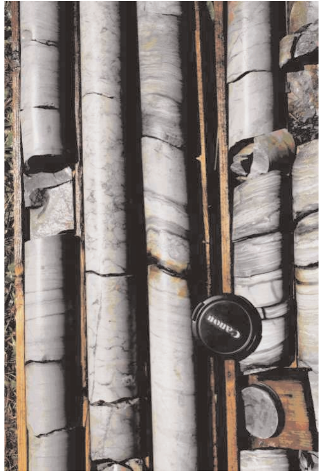
Plate 19. Dololaminite and burrow-mottled dolostone, Lower member, Aguathuna Formation, DDH RND 001, Port au Port Peninsula. Lens cap is 6 cm diameter.
