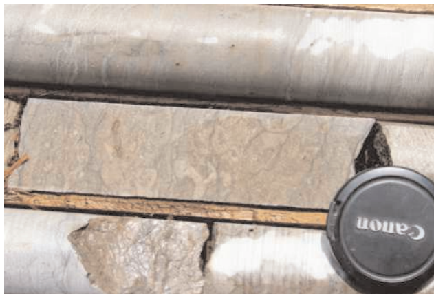
Plate 28. Skeletal intraclastic grainstone in the base of the Upper limestone member, Table Point Formation, DDH RND 001, Port au Port Peninsula. Lens cap is 6 cm diameter.
