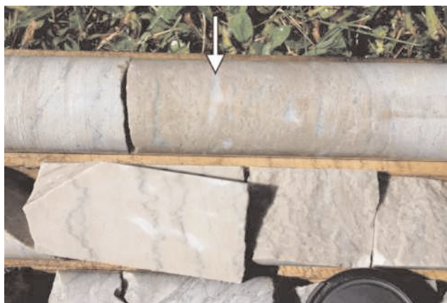
Plate 15. Peloidal, fenestral laminated limestone (upper run) of the Costa Bay Member, lying next to slabbed core of white, stylolitic, fine-grained peloidal grainstone. Note the spar-cemented stromatactoid cavities (arrow) in the laminite. Catoche Formation, DDH RND 001, Port au Port Peninsula. Lens cap is 6 cm diameter.
