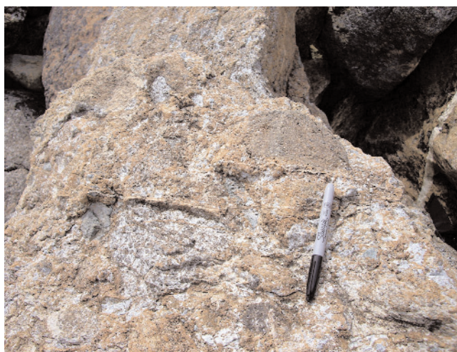
Plate 3. Listvenite appearance caused by the weathering of ankerite to limonite.
