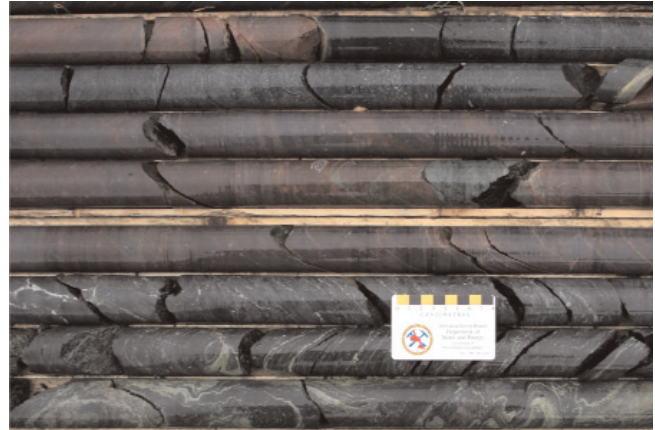
Plate 2. Locally developed folding of the penetrative fabric within the ash-flow tuff sequence.
