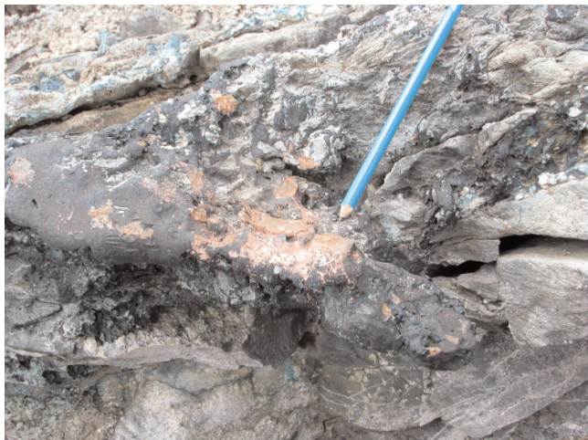
Plate 11. Tarnished and 'exposed' native copper nugget with malachite staining hosted in sheared quartz +/- carbonate vein, within chlorite-rich mafic volcanics. Mineralized veins are usually concordant to the fabric in host mafic volcanic. Individual nuggets have been measured up to 30 cm long and 10 cm wide at this locality. Pencil is 14 cm long (East Seal Lake showing No. 68, MODS number 13K/5/Cu020, UTM Coordinates 595389E/6017017N)
