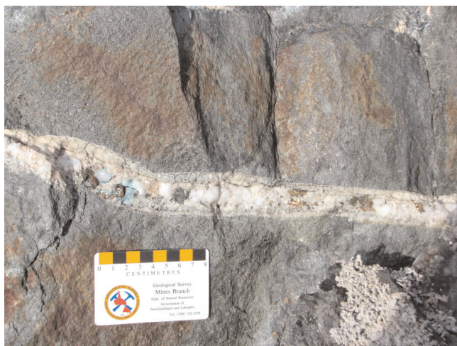
Plate 12. Chalcopyrite, minor bornite and malachite hosted in quartz + carbonate vein in a fine-grained diabase sill. Note zonation 'from coarse quartz' + minor carbonate crystals in core to fine-grained, predominantly carbonate + minor quartz at vein margins. North Whiskey Lake prospect, MODS number 13k/5/Cu003, (UTM coordinates 592098E/6015436N)
