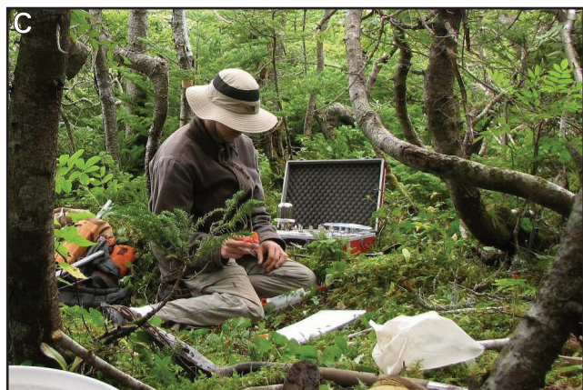
Plate 3. A) RS-230 spectrometer placed in soil-sampling pit for in-situ measurement. B) Insertion of soil-gas sampling probe. C) Measurement of radion ionizations with ERM2 electrometer.
