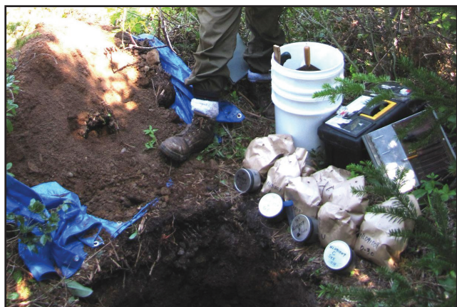
Plate 1. Samples collected from a single pit. The metal cans are used to collect samples for bulk-density and moisture-content determinations. The sample collected for Bacillus anthracis (anthrax) determination can be seen (in a clear plastic tube, with blue cap) between the second and third can.
