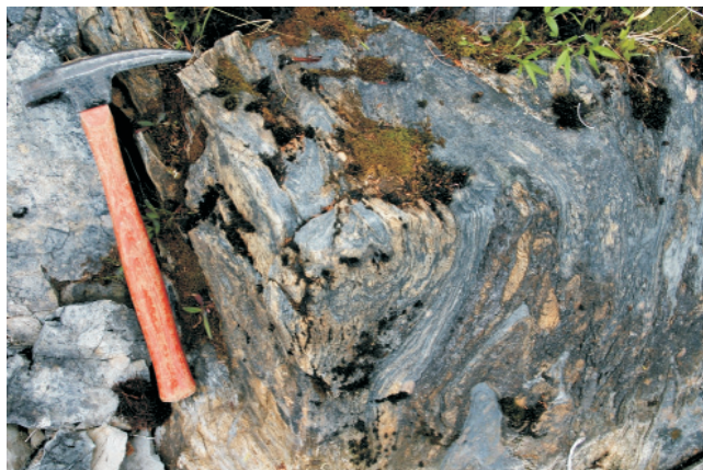
Plate 19. Folded limestone mylonite enclosing augen of dolostone lying in the footwall of the Smelt Pond thrust, the western shore of Smelt Pond. The original limestone belonged to Middle Cambrian March Point Formation. Hammer is 33 cm long.
