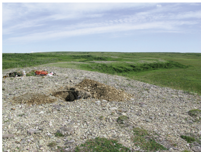
Plate 4. Gravel in hand-dug pit at top of 4- to 8-m-high esker in deposit 7, located 2 km east of Angels Cove.
