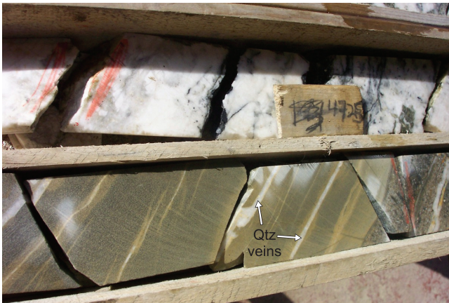
Plate 6. A flow-aligned, chilled margin of a TYPE-1 dyke cut by margin parallel, narrow white quartz veins. Core is 45 mm in diameter.
