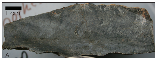
Plate 4. A) Hand sample of vein-hosted uranium mineralization that produced up to 60 000 counts per second in outcrop and assayed >1% U; B) Corresponding autoradiograph of the uranium mineralization (dark areas) within the hand sample. The autoradiograph procedure is summarized in Appendix A.
