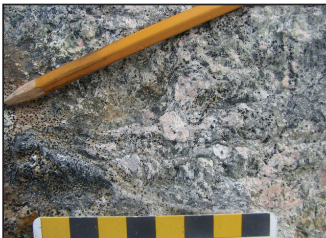
Plate 20. Recrystallized ‘tails’ on K-feldspar megacryst in submylonitic hornblende granodiorite. Asymmetry of the tail suggests a dextral shear sense. Unit 1, North Pole Brook Intrusive Suite, southern margin of Seal Lake Group, west of Dorothy Lake. (UTM coordinates 589655E/6008502N)
