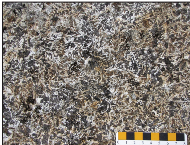
Plate 10. Medium-grained, massive, ophitic-textured gabbro, typically of the gabbro sill interiors. Subunit 4c, Wuchusk Lake Formation, south of Wuchusk Lake. (UTM coordinates 583704E/6025373N)
