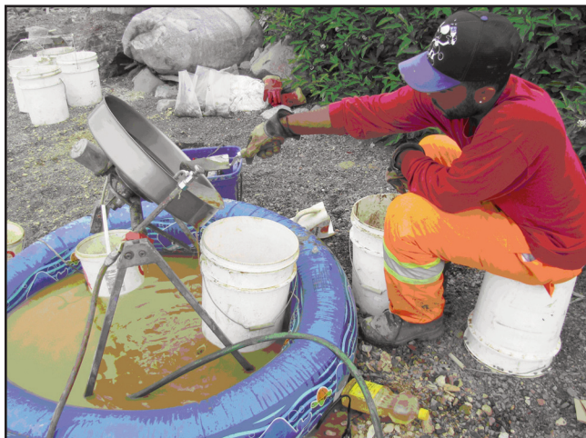
Plate 1. Panning a till sample using the Goldhound. The panned concentrate falls through the centre of the panner and accumulates in the small plastic pail. Light minerals are washed over the edge of the panner into the large pail along with water, which returns to the holding pool. Panning water is continually recycled by an electric pump.
