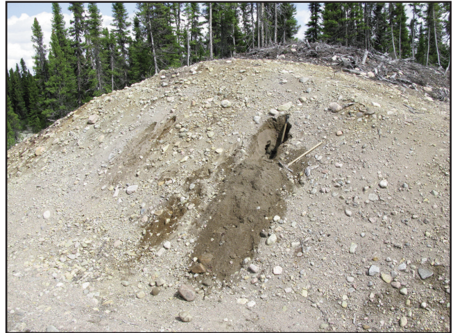
Plate 2. Sandy boulder gravel along a 3-m-high roadcut through esker; located in NTS map area 13B/10.
