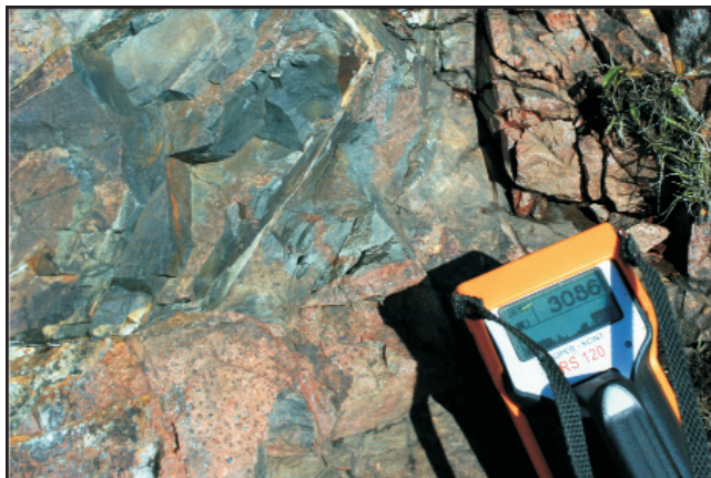
Plate 3. Localized uranium mineralization developed along the intrusive contact between black shale of the Inlet Group and quartz-porphyry of the St. Lawrence batholith at the Little Lawn River prospect.
