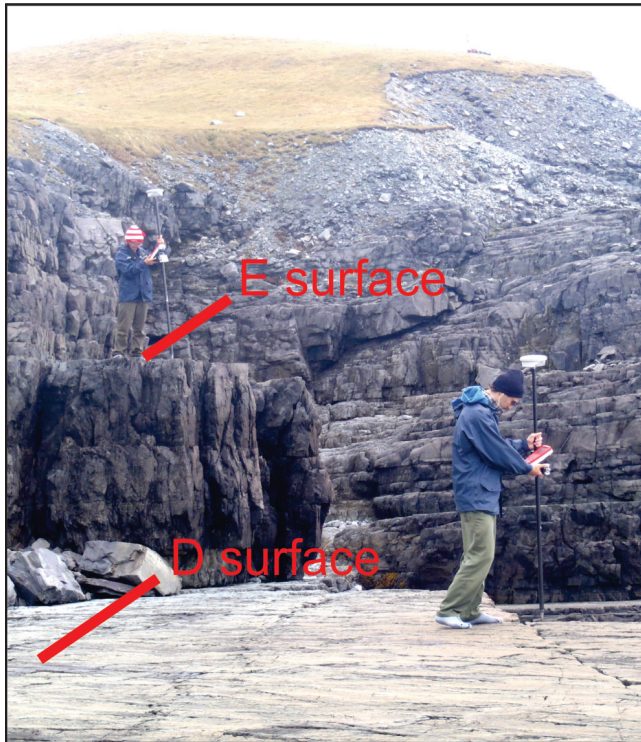
Plate 8. Coastal monitoring of D (foreground) and E fossil surfaces at Mistaken Point Ecological Reserve. Note eroding turfline with RTK base station setup in background. Coastal erosion is threatening to damage the 575 to 560 Ma Ediacaran fossils preserved in the mudstone and sandstone. Coastal monitoring will provide data onto the current rate of coastal erosion and the sensitivity of the area to change.
