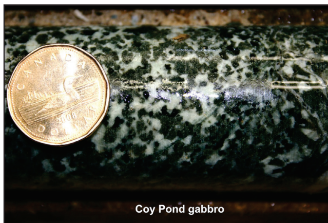
Plate 10. Massive, medium- to coarse-grained gabbro near the base of drillhole BO-09-22 (sample BO-09-22_168.2 m). Canadian $1 coin is 25 mm in diameter. This section of core was not assayed.
