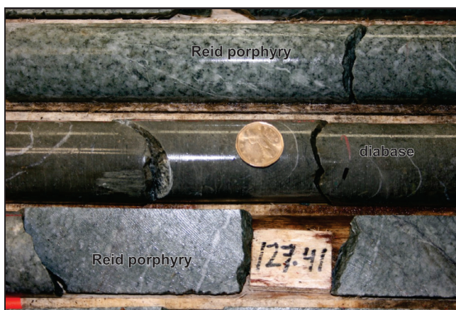
Plate 9. Fine-grained diabase dyke with thin quartz veins crosscuts quartz-plagioclase porphyry in diamond-drill hole BO-09-17 (sample BO-09-17_125.9 m). Canadian $1 coin is 25 mm in diameter. The diabase was not assayed.
