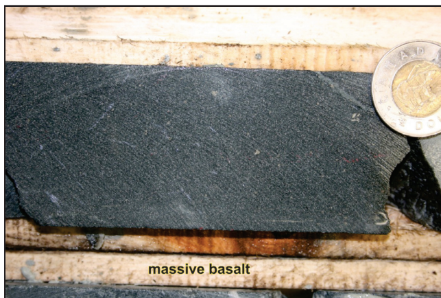
Plate 1. Massive, fine-grained pyritic basalt from the top of drillhole BO-09-17 (sample BO-09-17_7.13 m). This intersection yielded an assay of <5 ppb Au. The $2 coin is 28 mm in diameter.
