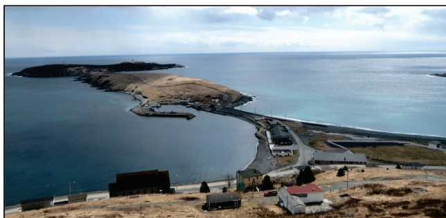
Plate 4. The main beach and tombolo in Ferryland (Figure 1, Site #310) are highly sensitive to erosion and flooding caused by combination of local factors; the tombolo has a low elevation, is narrow, is frequently exposed to storm surges and large waves, and lacks natural protection from sea ice (Catto, 2012a, b). The area has a history of flood events, which have caused extensive and repeated damage to the road leading out to the headland. Photo credit: Eric Watton.
