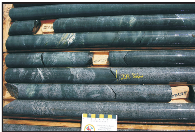
Plate 12. Photograph highlighting the sharp intrusive contact between the foliated metavolcanic country rock and undeformed medium-grained granodiorite to quartz monzonite at the Jacques Lake deposit (DDH JL07-58A; 230 m depth).
