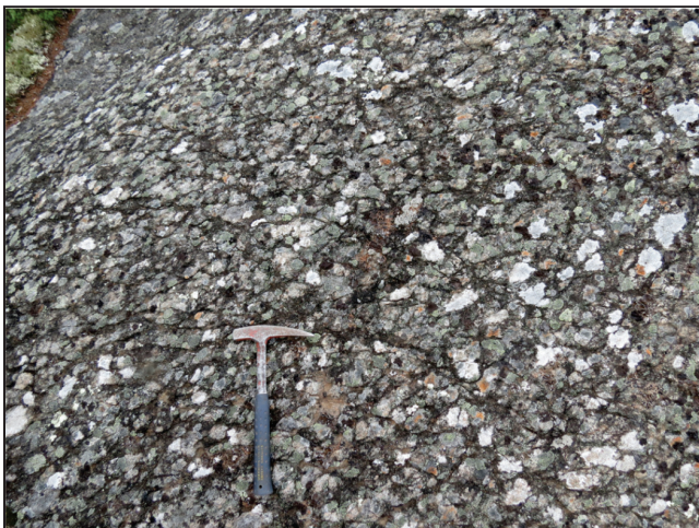
Plate 5. Massive to weakly foliated, porphyritic pyroxenite of the ultramafic sill in the southern study area (sample 13VN127A02). Orthopyroxenes (grey-green-weathering crystals) are interpreted as relict igneous oikocrysts. White patches are lichen-covered oikocrysts.
