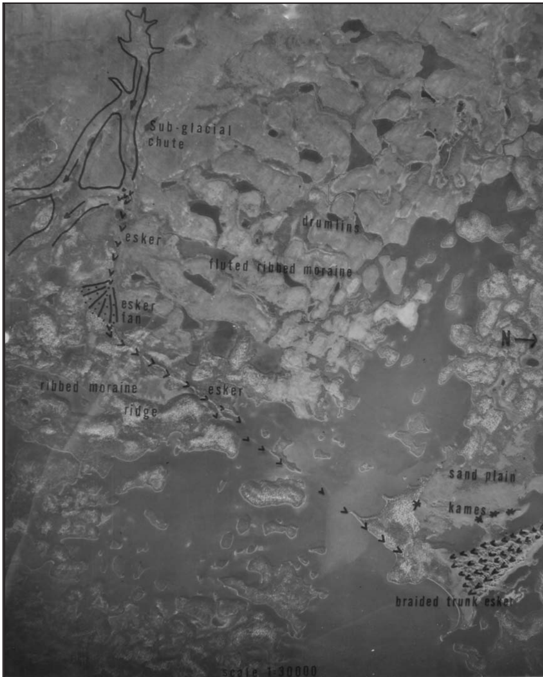
Figure 5. Aerial photograph reproduced from Cowan (1967, Plate 6, page 49) showing the relationship between subglacial chutes, eskers, moraines and outwash in the Shoal Lake area.
