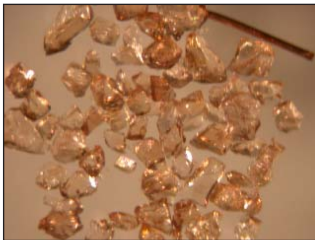
Figure 5. U–Pb concordia diagram (left) for two fractions of zircons, like those shown in the photograph (right), separated from the pyroxene leucodiorite (leuconorite). See Table 1 for characteristics of analyzed fractions selected from the pictured zircons. Wire is 100 microns (0.1 mm) across.
