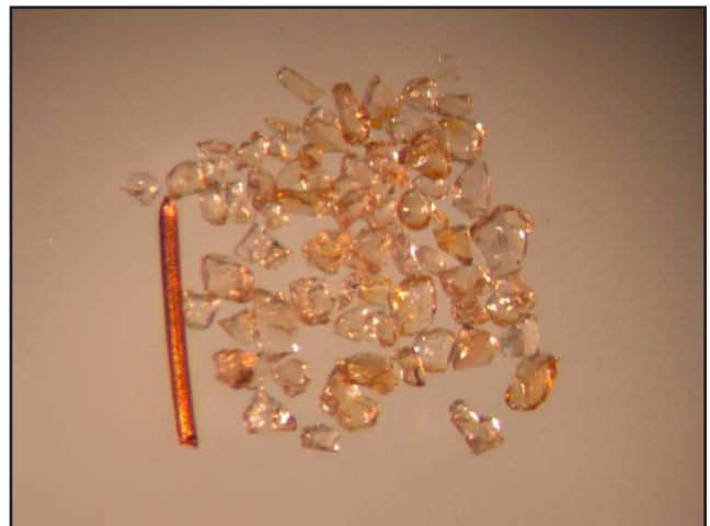
Figure 6. U–Pb concordia plot (left) for isotopic data from two fractions of the zircon grains, selected from those shown in the photograph (right), from the “maggoty” meladorite (melanorite). Wire used for scale in photograph is 100 microns (0.1 mm) across.
