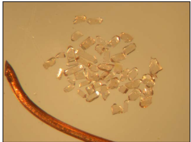
Figure 4. U–Pb concordia diagram data plot for the leucogranite dyke (left) and a photo of the population of analyzed zircons (right) from which the age was obtained. Dyke crosscuts the leuconorite intrusion from the same area (see Figure 3). See Table 1 for characteristics of analyzed fractions selected from the pictured zircons. Wire used for scale is 100 microns (0.1 mm) in diameter.
