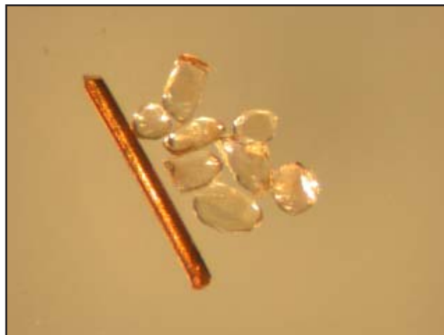
Figure 7. U–Pb concordia diagram (left) derived from isotopic analyses of two fractions of zircons, selected from the small group shown in the photograph (right), separated from the pyroxene–olivine granite (charnockite). Wire for scale in photograph is 100 microns (0.1 mm) across.
