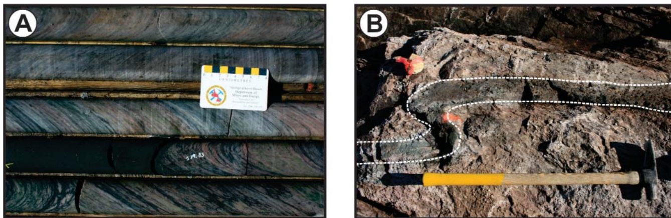
Plate 3. A) Locally developed mylonitic texture within the crystal tuff unit, crosscut by a post-kinematic mafic dyke; DDH M07-075, ~ 380 m depth; B) Folded mafic dyke crosscutting the quartz- and feldspar-phyric metarhyolite dyke within the main exploration trench of the Michelin deposit.
