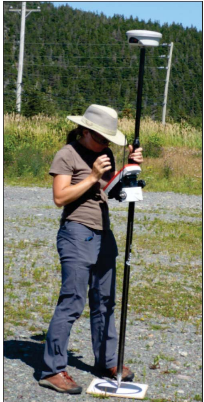
Plate 5. The Ground Control Points (GCPs) are of 30 by 30 cm black and white targets mounted on plywood. The operator is surveying the centre point of the GCP with the roving receiver of the RTK system.
