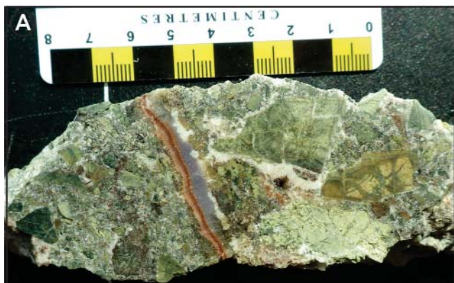
Plate 1. Brecciation of host rocks representing the first phase of hydrothermal activity. A) Strongly altered rhyolite breccia cut by a fluorite vein; B) Moderately altered rhyolite clasts in strongly altered matrix.
