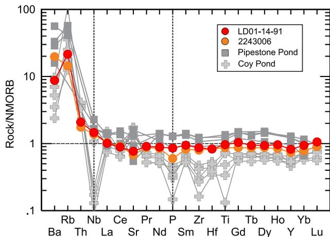
**Figure 5.** NMORB normalized extended incompatible trace-element diagram comparing samples LD01-14-91 and 2243006 with historical data for lavas of the Pipestone Pond complex (Jenner and Swinden, 1993) and the Coy Pond Complex (Sandeman et al., 2012).
