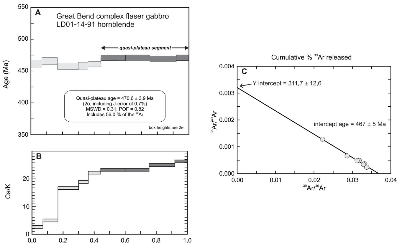
**Figure 3.** A)  $^{40}\text{Ar}/^{39}\text{Ar}$  age spectrum for hornblende from specimen LD01-14-91; B) Ca/K vs. cumulative fraction of  $^{39}\text{Ar}$  released showing the relatively consistent and high Ca/K for the quasi-plateau steps; C)  $^{36}\text{Ar}/^{40}\text{Ar}$  vs.  $^{39}\text{Ar}/^{40}\text{Ar}$  inverse isochron plot for the sample.
