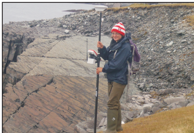
Real Time Kinematic surveying at Mistaken Point Ecological Reserve to monitor rates of coastal erosion.
