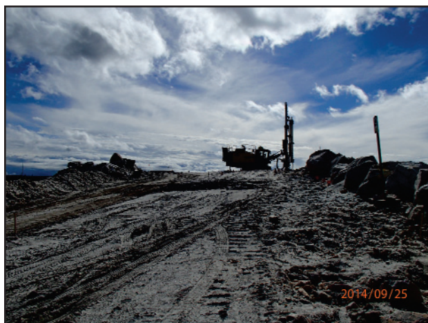
IOC drilling in preparation of blasting to reduce pit slopes during rehabilitation of the Leila Wynn dolomite mine.
