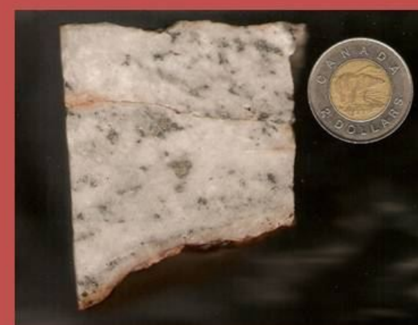
Pyrite and galena, with lesser amounts of chalcopyrite and sphalerite, make up the sulphide mineral assemblage.
