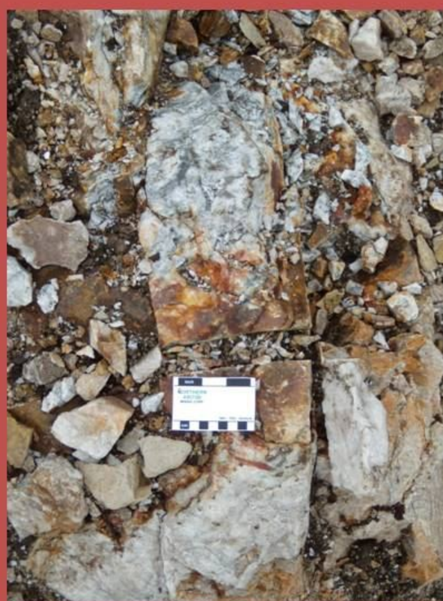
Outcrop photo of the Thor vein. A 1.5 to 8 meter wide quartz-sulphide vein which dips gently to the south and closely parallels a carbonate-altered mafic dyke.
