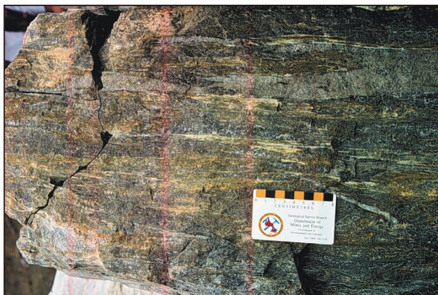
Plate 60. Typical banded silicified and sericitic, sulphide-bearing schist from the Footwall Zone, Rambler Main Mine.
