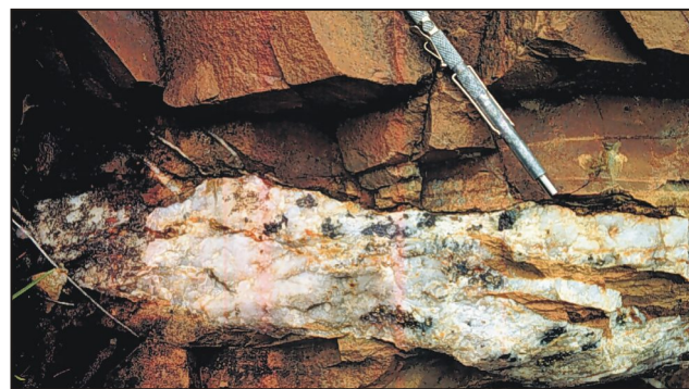
Plate 43. Pyrite-chalcopyrite-tetrahedrite-bearing quartz vein, Penny Cove showing. Grab samples collected from this vein have assayed up to 5.979 g/t Au.
