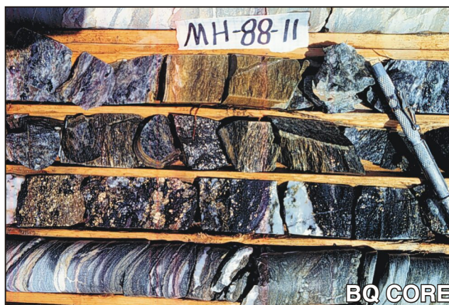
Plate 52. Closeup of mineralized core, diamond-drillhole MH-11-88, Goldenville Mine. Section exhibits quartz veining cutting deformed oxide-facies iron formation. Pyrite replacing magnetite mantles the quartz veining. This particular section assayed 12.89 g/t Au over 1.8 m.
