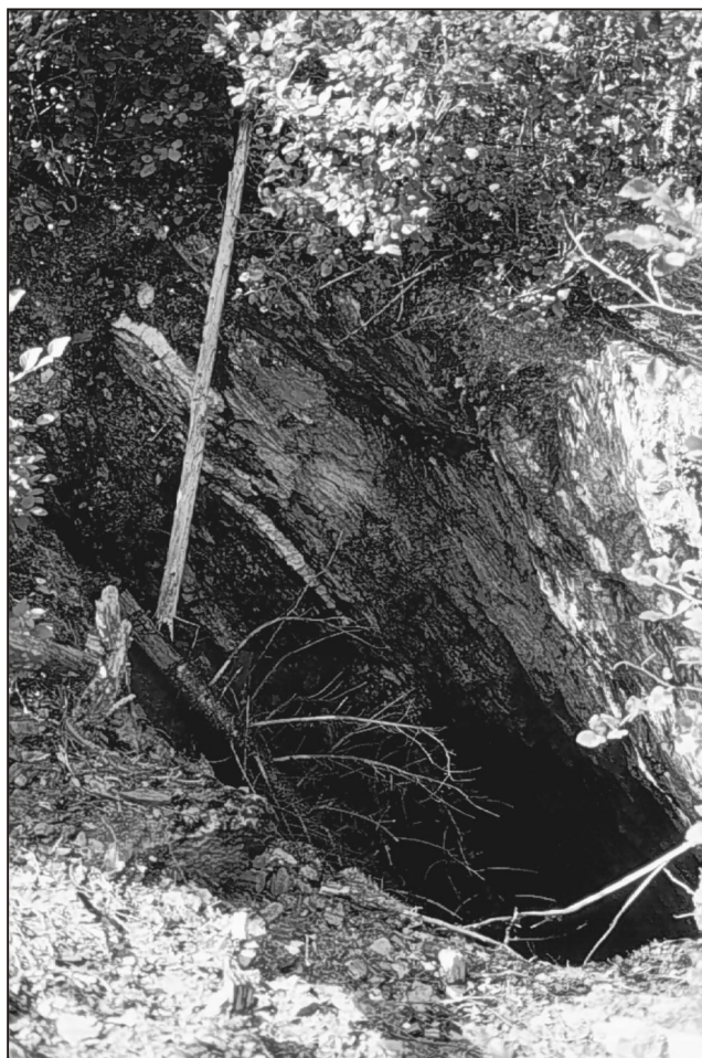
Plate 50. North Shaft, Goldenville Mine area. Mylonitized volcanic breccia is exposed in the old shaft. The shear zone contain weakly pyritic quartz veins; grab samples of these veins assay up to 3 g/t Au.
