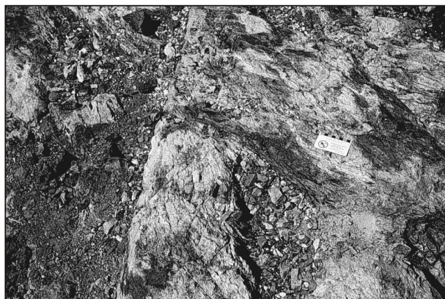
Plate 45. Pyrite-bearing fractures developed within tonalite, Corkscrew prospect. A grab sample collected by the author assayed 5.83 g/t Au.
