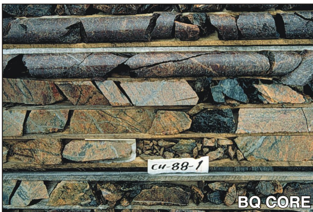
Plate 20. Diamond-drillhole CH-88-01 that intersected sericitized and quartz veined felsic crystal tuff of the Mic Mac Lake group, Crow Hill North. Note the unaltered maroon felsic crystal tuff at the top of the photograph.
