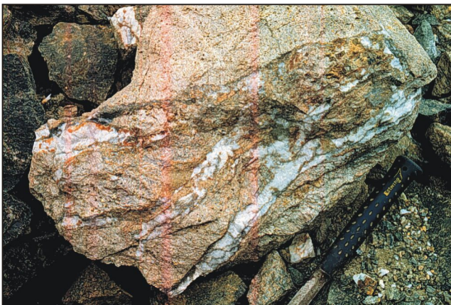
Plate 54. Typical Stog'er Tight ore composed of red albite-pyrite cut by milky-white quartz-albite-ankerite veins. Note the coarse disseminated euhedral pyrite within the altered gabbro.
