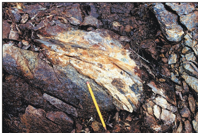
Plate 70. Porcelain white, coarse-grained magnesite–dolomite–talc vein, containing small clots of magnetite, cutting talc–carbonate altered ultramafic rocks, Fox Pond #1 showing.
