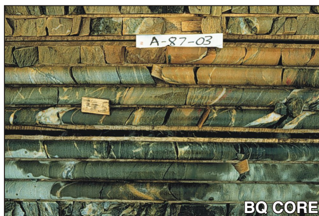
Plate 24. Diamond-drillhole A-87-03 showing the gradational nature of the carbonitization, Albatross prospect.
