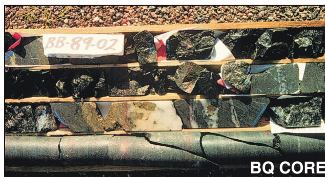
Plate 63. Coarse pyrite-bearing quartz vein developed at the contact between a gabbroic dyke and mafic volcanic rocks, diamond-drillhole BB-89-02 Brass Buckle prospect. The 30 cm interval assayed 17.25 g/t Au.
