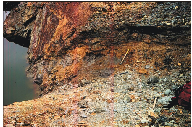
Plate 59. Section through the Rambler Main Zone as exposed in the Footwall Zone open pit. The grey rocks in the foreground are the silicified footwall. The massive sulphide outcrops next to the hammer. The sulphide body is intruded here by a massive diorite dyke (centre of photograph).
