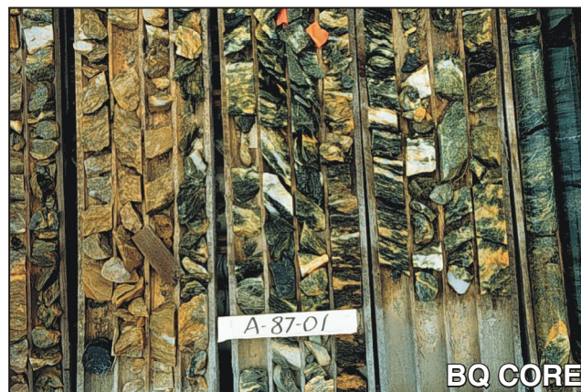
Plate 26. Example of the chlorite–ankerite alteration assemblage, diamond-drillhole A-87-01, Albatross prospect.
