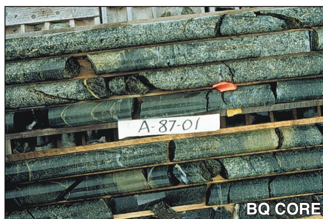
Plate 23. Medium-to coarse-grained gabbro of the Advocate Complex cut by diabase dykes, diamond-drillhole A-87-01, Albatross prospect. Note zones of epidotization.
