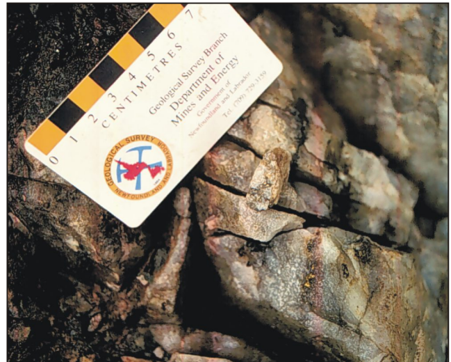
Plate 58. Closeup of the Stuckey Vein illustrating the grey, sugary-textured quartz. Gold is visible in the small quartz fragment at the centre of the photograph just below and to the right of the scale. A small clot of chalcopyrite is present at the bottom of the photograph.
