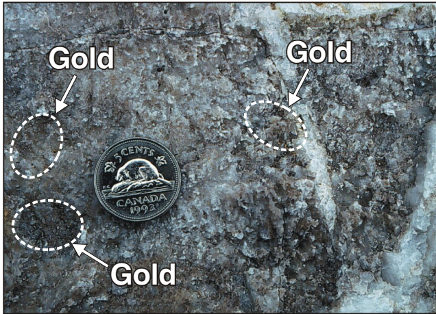
Plate 39. Closeup of a mineralized vein margin, Juliet South Zone. The pitted surface is a vein margin containing fine flecks of gold and small patches of green sericite.
