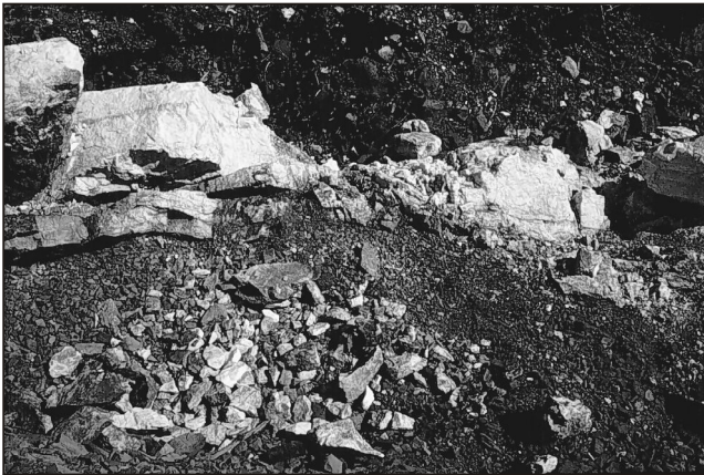
Plate 37. Oblique strike-slip fault that offsets the Juliet South Zone. Dextral offset on the vein is approximately 1 m.
