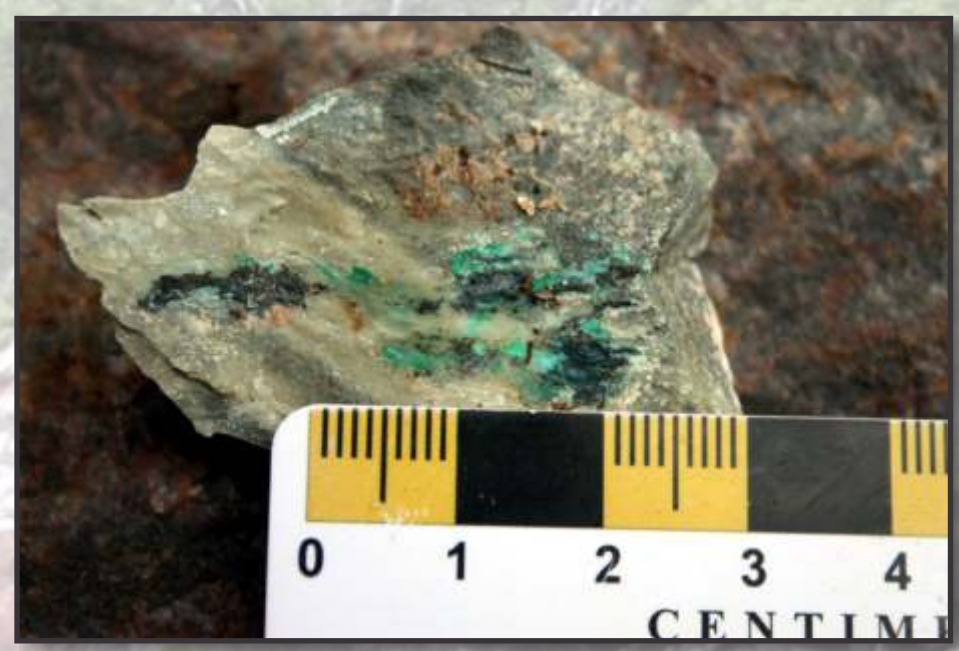
Chalcocite and malachite mineralization in the Blue Point horizon, Crown Hill Fm., west of Little Heart's Ease.
