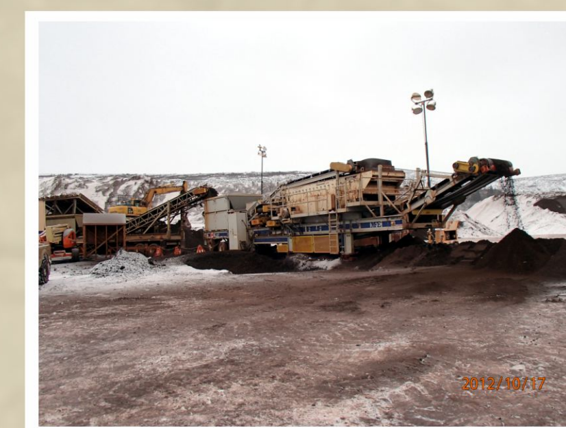
Screening direct rail iron ore (DRO) from Labrador Iron Mines Ltd.'s James North Mine.
