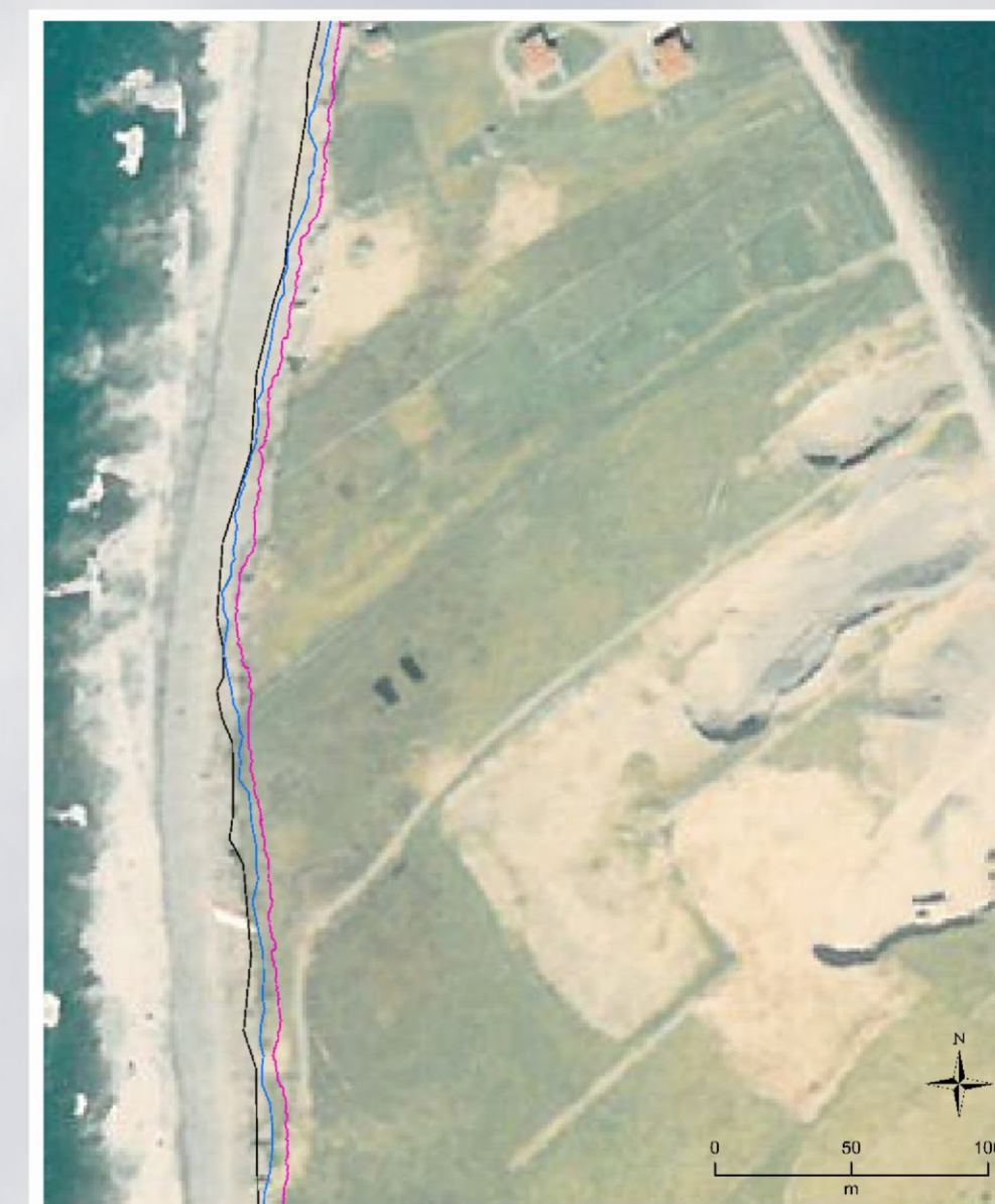
Cliff top in 1991 (black), 2000 (blue) and 2012 (pink) superimposed on an airphoto. Cliff erosion varies between 0.5 m/a to 1 m/a.
