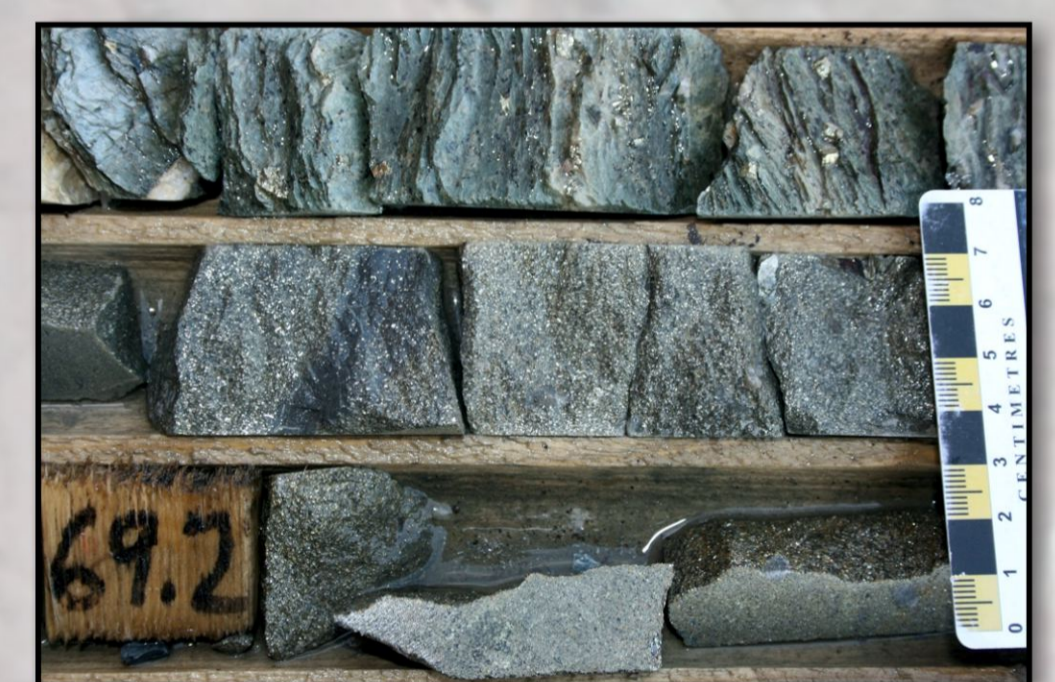
Massive sulphides at Long Lake, grading: 2.7% Cu, 1.1% Pb, 23.6% Zn, 45 g/t Ag and 0.7 g/t Au.
