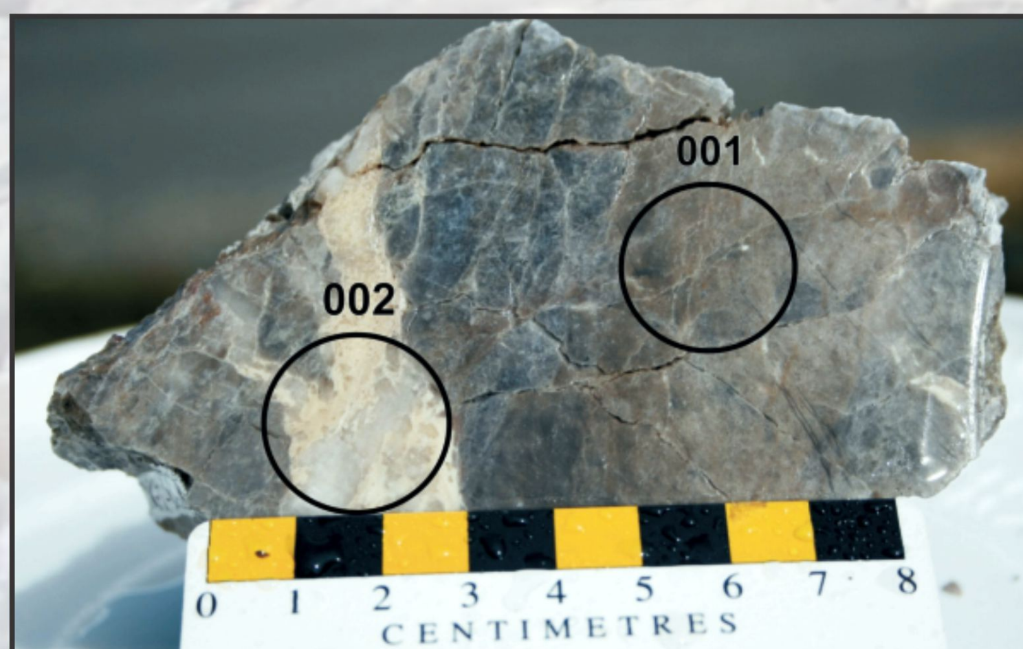
Altered sample from epithermal gold mineralization at Rattle Brook, northern Burin Peninsula, showing the spectrometer identifications of key alteration minerals such as illite and dickite.
