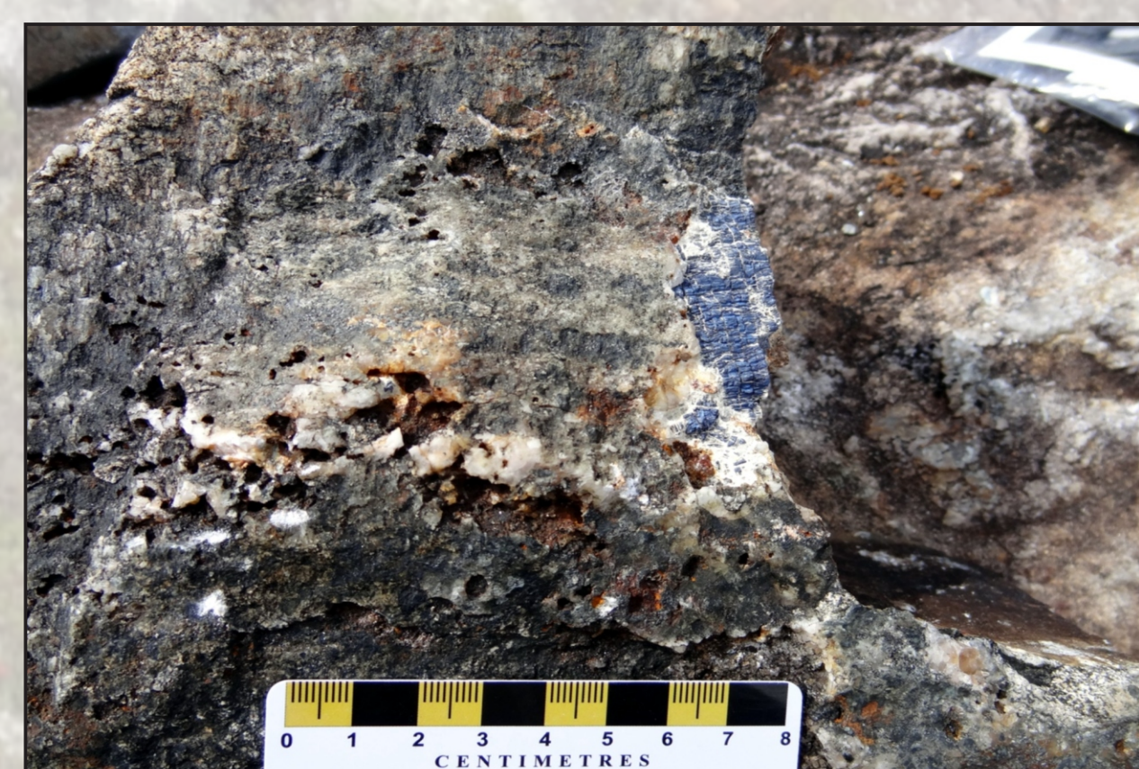
Galena crystals in quartz + carbonate vein cutting migmatitic paragneiss of the Ashuanipi Complex. The occurrence consists of two sets of late veins containing 1-3% coarse galena crystals and fine-grained disseminations. The veins are located immediately below the unconformity with arenite and conglomerate of the Mesoproterozoic Wishart Formation of the Labrador Trough.
