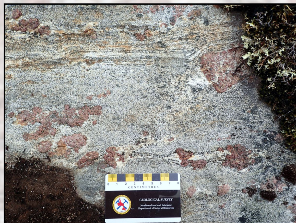
Well-banded metasedimentary gneiss enclave in garnet-dominant granodiorite diatexite. The slight warping of the S 1 migmatitic fabric around the large inclusion-rich garnet at top right suggests the diatexite (and garnet growth) formed pre- to syn-D 1 deformation.
