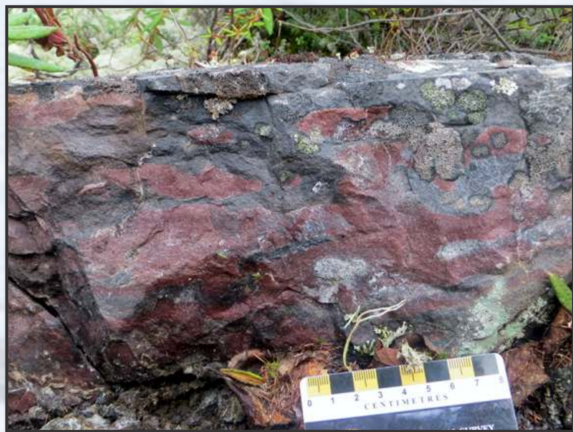
Taconite ore with irregular bands of red chert and grey magnetite (Labmag deposit)
