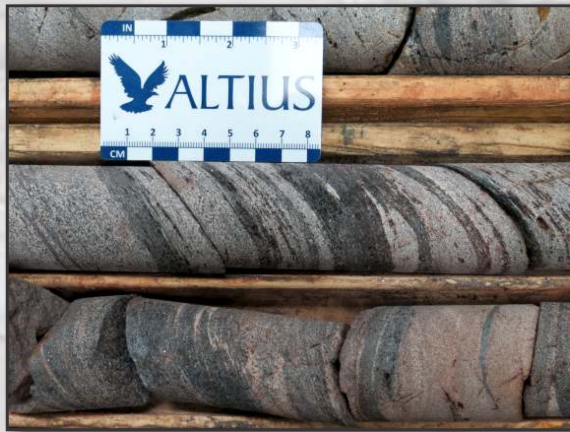
Metataconite ore with bands of coarse grained quartz and hematite (Julienne Lake deposit)
